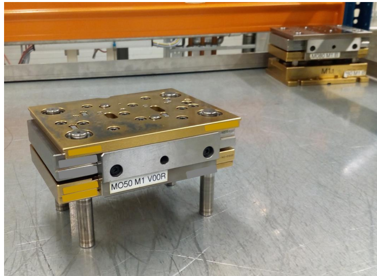
Figure 12: Upper part of a cold-forming tool-module (foreground) and a complete tool-module (background)
