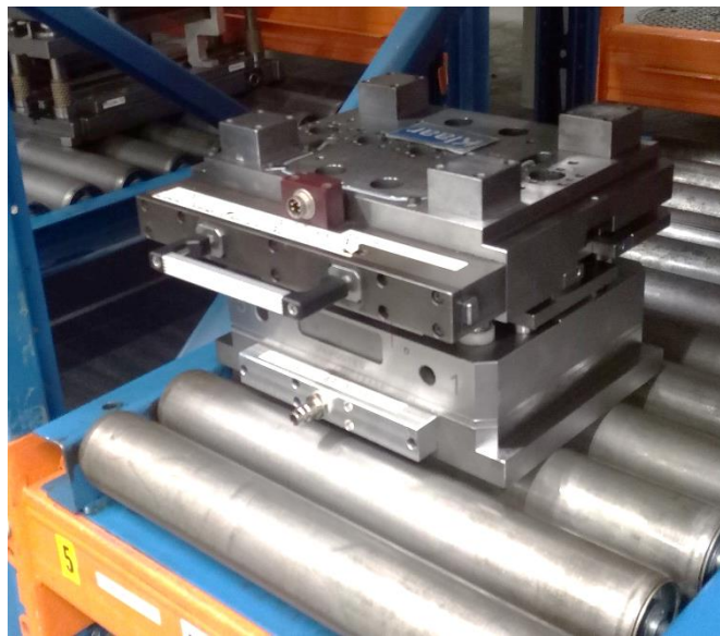
Figure 13: 5-fold cutting-out tool, ready for manufacturing
