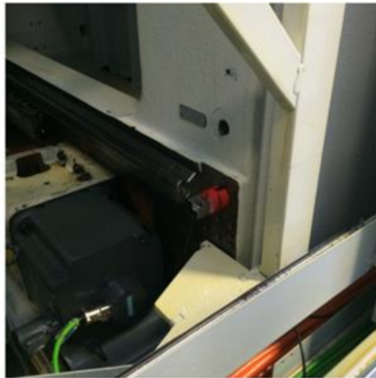
Figure 35: Position of the Artis GEM 3D accelerometer positioned on the casting next to the X-axis rail
